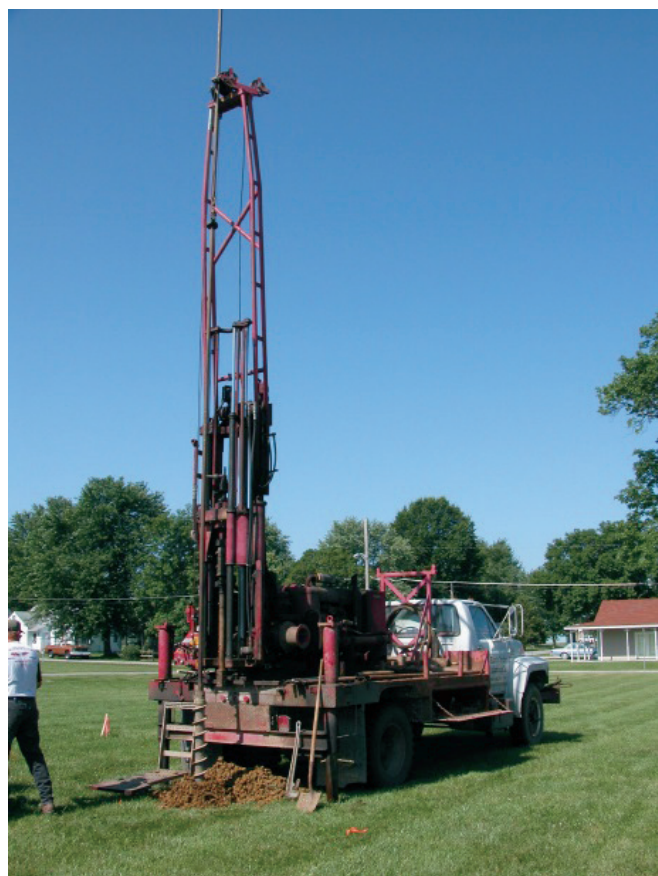
Auger Drilling Operation Figure 2-7
